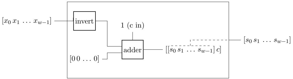
The “invert” circuit flips each incoming wire by using a separate NOT gate for each wire:
