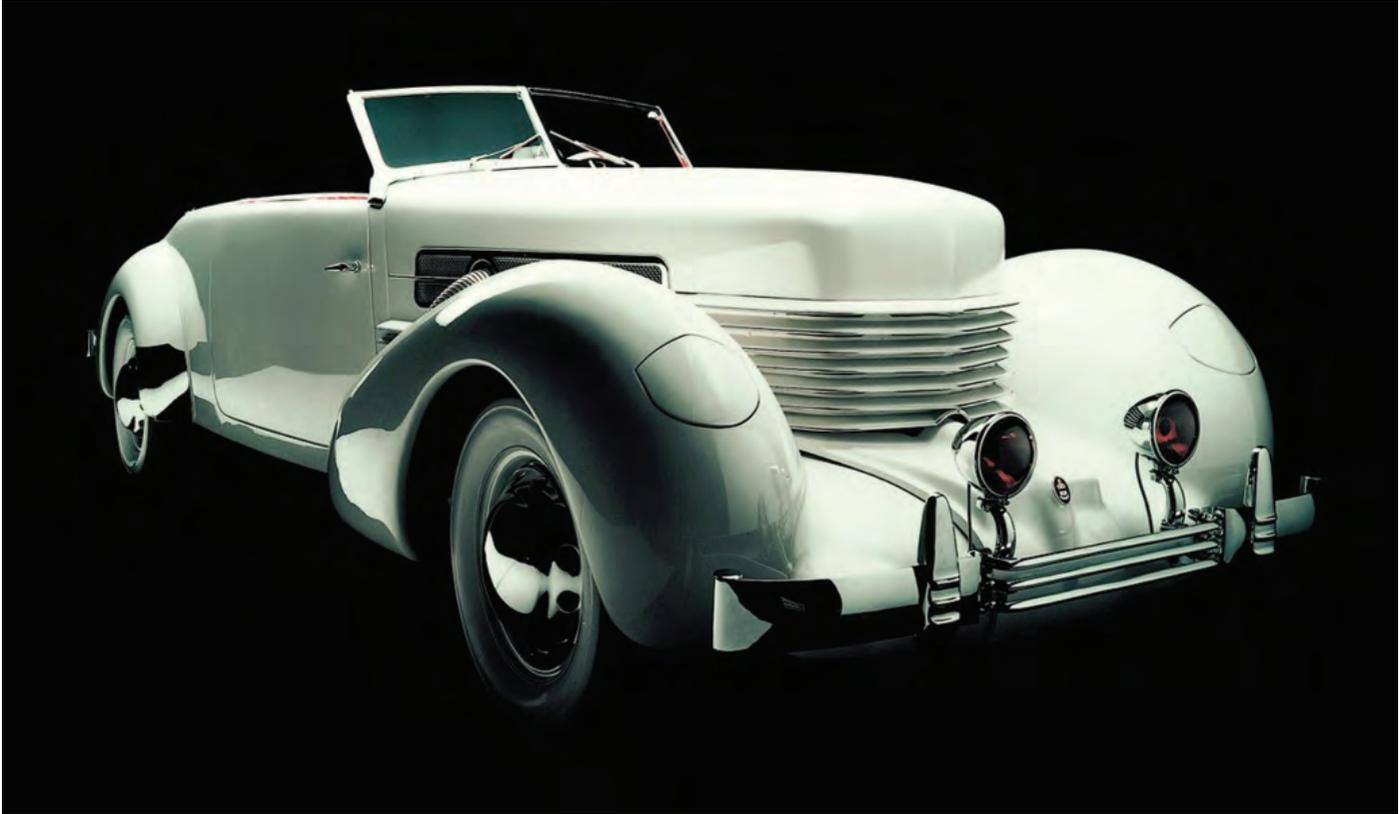
The revolutionary Cord 810 by Gordon W. Buehrig was a vehicle ahead of its time, full of novel technical features such as front-wheel drive and retractable headlights. This model, an example of which was owned by the American architect Frank Lloyd Wright, was presented at the New York Auto Show in 1935, an exhibition visited by Le Corbusier during his stay in the United States. According to *Autocar* magazine, in 1936 it was "currently the least orthodox automobile in the world."
