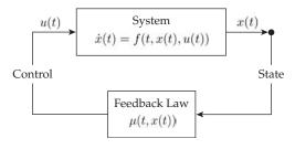
**Figure 1.3** Feedback control system.
