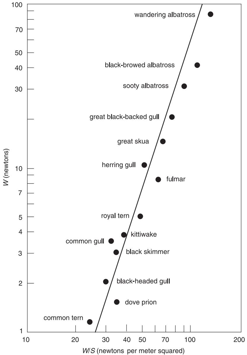
**Figure 1** The relation between weight and wing loading represented in a proportional diagram. When the weight increases by a factor of 100, the value of  $W/S$  increases by a factor of 5 and the airspeed by a factor of more than 2.
