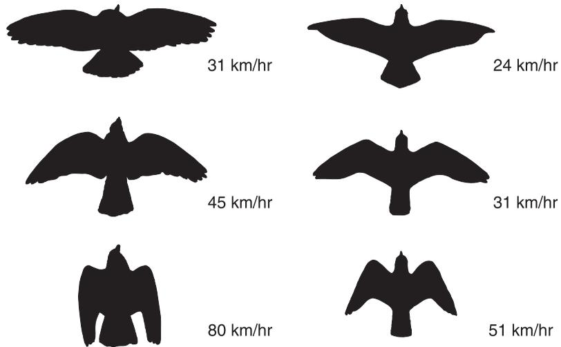
**Figure 3** Birds progressively fold their wings as their speed increases. On the left is a pigeon, on the right a falcon. At high speeds, fully spread wings generate unnecessary drag. This can be avoided by reducing the wing area.
