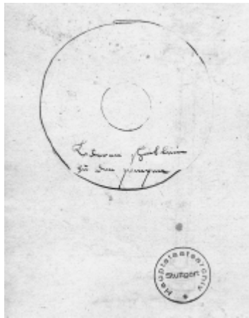
Figure 1.13. Documentation of the size of a leather disc for sealing pistons in a pump cylinder. Drawing by Heinrich Schickhardt, 1603. (Stuttgart, HStA, N220 T150, all rights reserved.)
