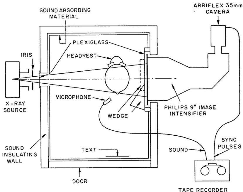
**Figure 2.1** Schematic representation of the cineradiographic and sound-recording facility.
