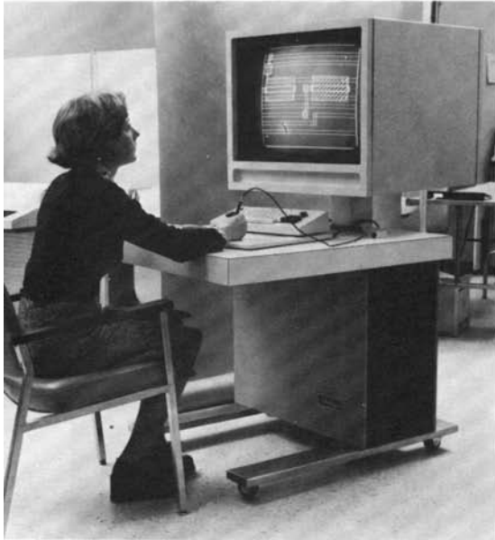
The microcircuit is laid out with the aid of a computer. Sections of the large-scale integrated circuit can be scrutinized and modified with a light pen on a visual display unit. Photo courtesy of Applicon
