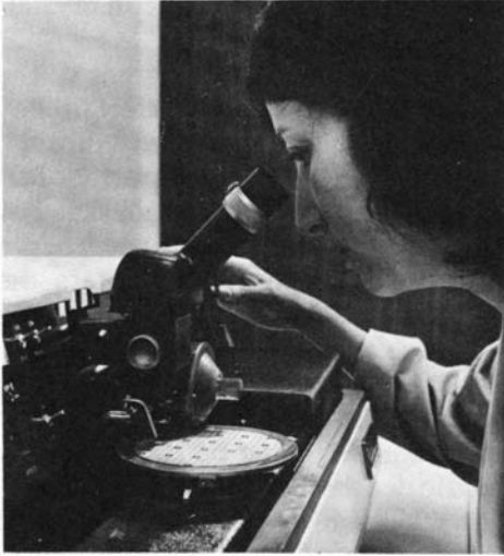
When the chips have been built up on the wafer, grooves are cut into the surface, prior to breaking the wafer into individual dice. Photo by Jon Brenneis
