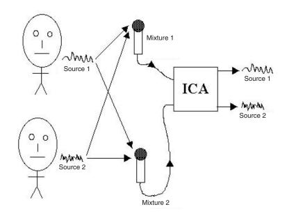
ICA in a nutshell. If two people speak at the same time in a room containing two microphones then the output of each microphone is a *mixture* of two voice signals. Given these two *signal mixtures*, ICA can recover the two original voices or *source signals*. This example uses speech, but ICA can extract source signals from any set of two or more measured signal mixtures, where each signal mixture is assumed to consist of a mixture of source signals (see text).
