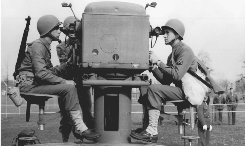
Figure 1.5 M-9 gun director, tracking head with operators. One follows the target in elevation, the other in azimuth. The unit and the operators rotate with azimuth tracking. (AT&T Archives)
