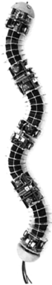
Figure 1.10 Snake robot developed at the Fraunhofer Institute for Autonomous Intelligent Systems in Germany (photograph courtesy of the Fraunhofer Institute)
