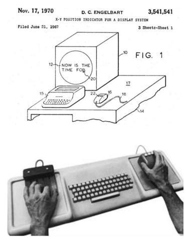
Figure 1.8 Image from the original mouse patent, filed in 1967 by Douglas Engelbart, showing it controlling a "tracking point" (cursor) on the screen, and a still image from Engelbart's public demonstration of his system in 1968 in which he is using the mouse with his right hand and a chording system similar to command keys with his left hand.
